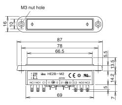
• M3 nuts are supplied with the HE2B enabling switch.
